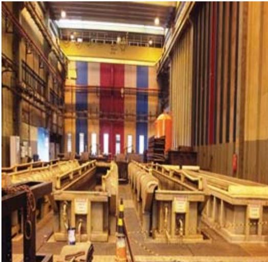
Fig.2 Hydrochloric acid tanks for pickling
