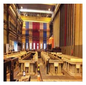
Fig.2 Hydrochloric acid tanks for pickling Source: Setaviso Engineering [2013]
