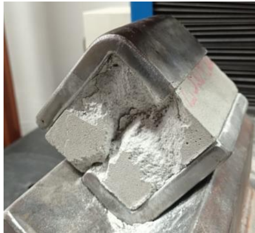
Figure 3 – Specimen ruptured by shear.
