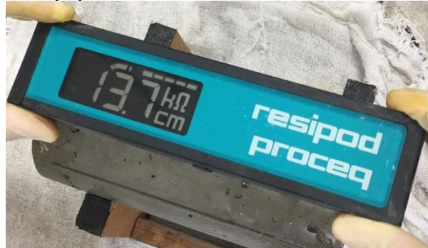
Figure 5 – Equipment used to test surface electrical resistivity.
