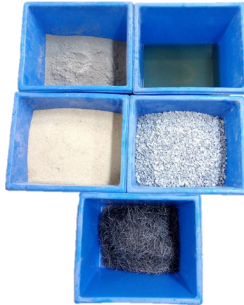
Figure 3: Materials used in preparation of concrete.
